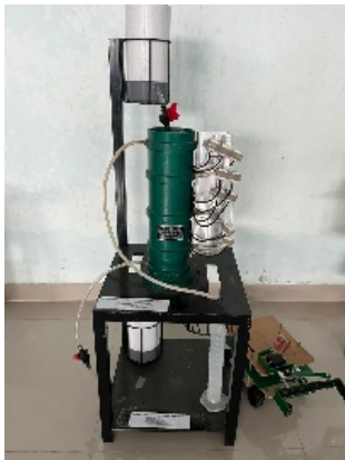
Rancang Bangun Smart Portable Soil Permeability Test
